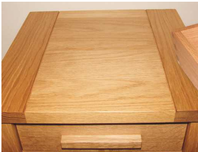
▲ Pic.7 The top's breadboard construction was detailed to match the 3mm grooves on the side rails
